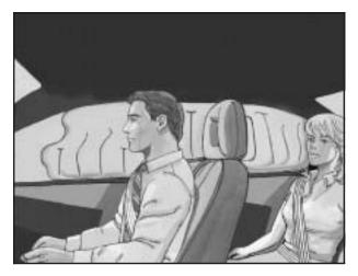
If your vehicle has a roof-mounted airbag for the right front passenger and the person directly behind that passenger, it is located in the ceiling above the side windows.
